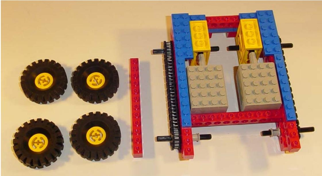
Add 4 large wheels and one 1x12 red beam across the top of the robot as shown here:
