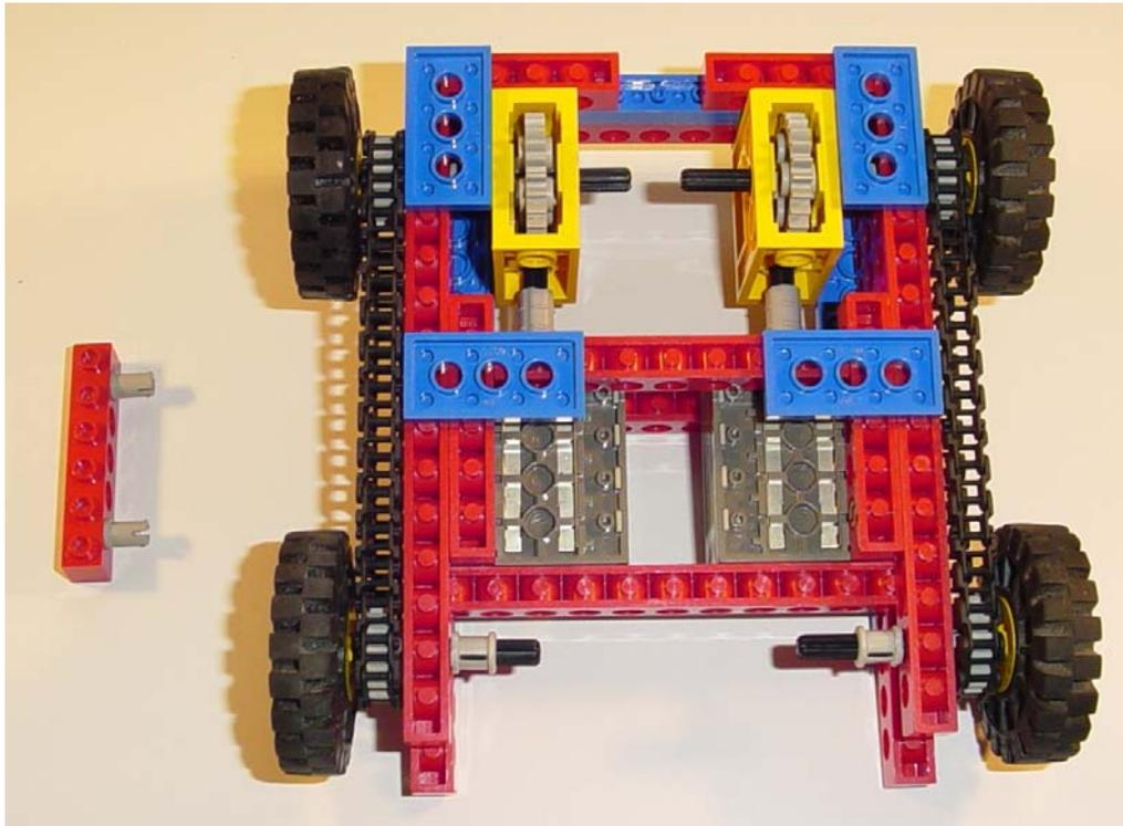
The grey pins go into each end of the shorter red beam, and that beam connects the top and bottom red beams to help hold the motors in place giving the robot additional strength. A photo of the completed robot is on the next page.
